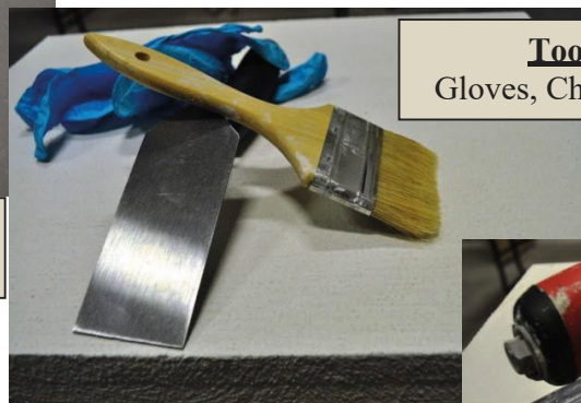
Tools Needed for Brush Coats: Gloves and a Chip Brush
