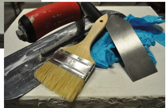
Tools Needed for Trowel Coats: Gloves, Chip Brush, Margin & Pool Trowel
